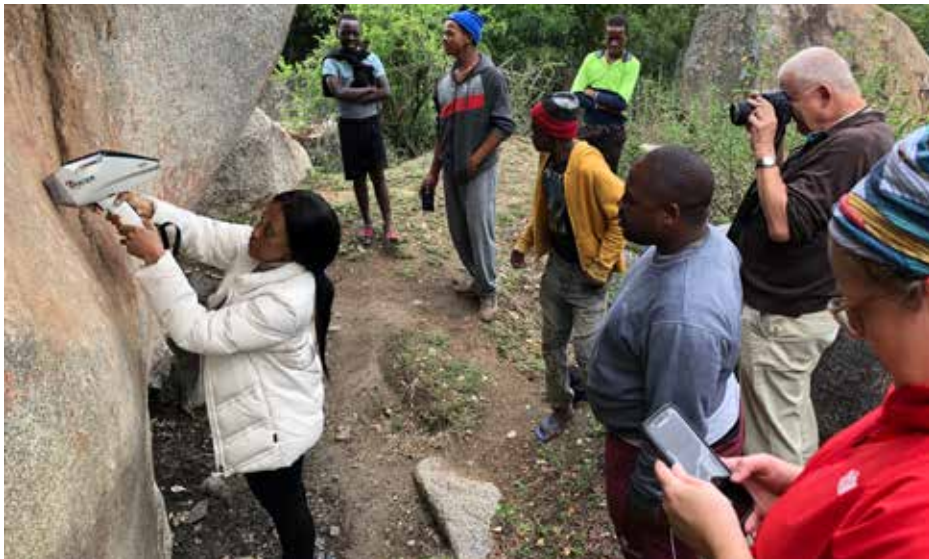
Conducting XRF analysis to determine the elemental composition of the rock art at a Late Stone Age site (Photo: L. Ehlers)
